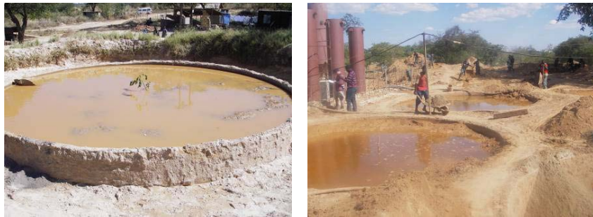
Fig. 6.4 - Vat leach at a milling center in Zimbabwe
