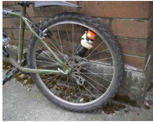
Fig. 5.13 – Mercury filter made of PVC cups attached to a bicycle wheel centrifuge
