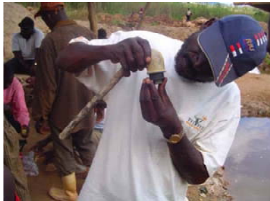
Fig. 5.38 - Miner closing an RHYP pipe retort in Mozambique. Note that the pipe plug crucible is threaded directly into the elbow.
