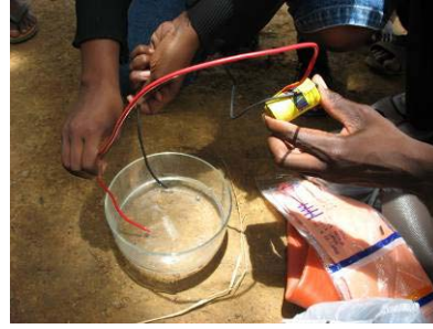
Fig. 5.4 – Miner activating mercury using a radio battery; the process takes about 10 - 20 minutes
