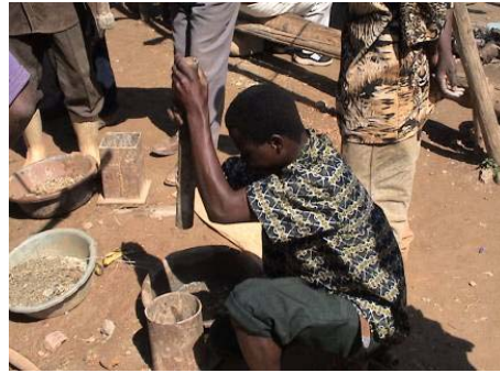
Fig. 3.22 – Miner crushing and grinding with mortar and pestle in Mozambique
