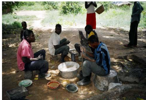
Fig. 3.20 – Miners in Zimbabwe grinding with mortar and pestle, and screening manually
