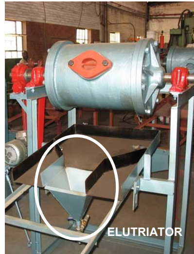
Fig. 5.9 – ABJ amalgamation barrel with short elutriator (copper plate not shown)
