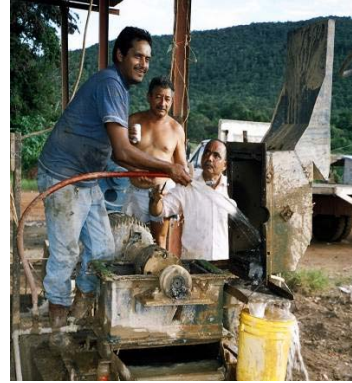
Fig. 3.10 – Miner washing a hammer mill after operation to remove gold stuck inside the mill (Venezuela)
