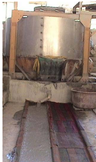
Fig. 4.7 – Ground ore from a Chilean pan feeding alternating sluice boxes with carpet (Ecuador)
