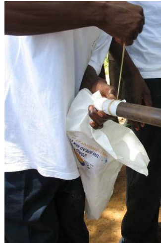
Fig. 5.41 – Making a “mvuto”: a steel pipe is inserted through a hole in the corner of a plastic bag and tied with string
