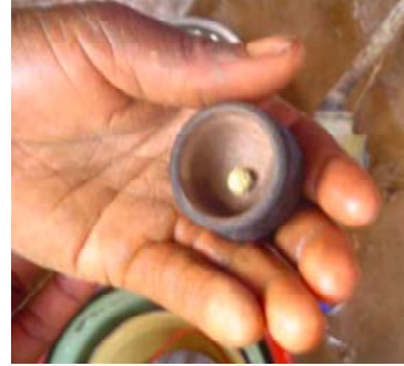
Fig. 5.24 - Miner showing retorted gold ( doré ) in the crucible (a hollow pipe end cap) of a RHYP retort
