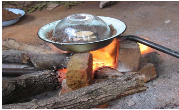
Fig. 5.31 – Kitchen-bowl retort on a bonfire in Zimbabwe (using a “mvuto” blower).
