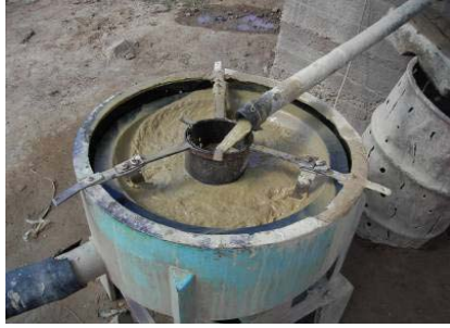
Fig. 4.13 – ABJ centrifuge operating in Zimbabwe
