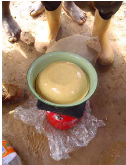
Fig. 5.33 – Kitchen-bowl retort using a metallic bowl instead a glass bowl as cover and a kerosene stove for heating; a metallic cover cools down faster than glass
