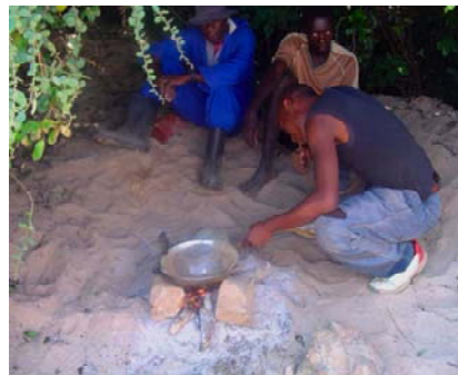
Fig. 5.30 – Zimbabwean miners using the kitchen-bowl retort on a bonfire
