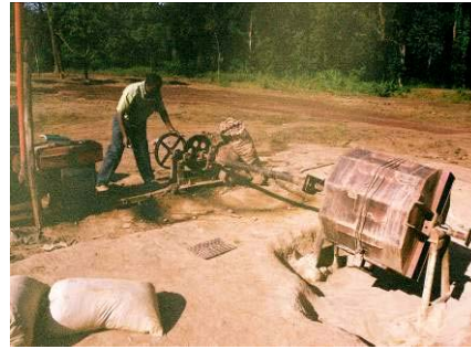
Fig. 3.18 - Diesel driven octagonal welded dry ball mill in Tanzania
