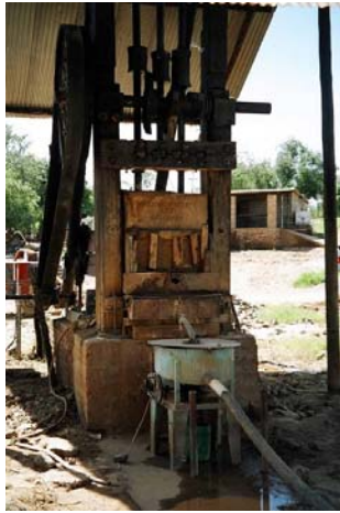
Fig. 3.11 – Three-stamp mill in Zimbabwe discharging crushed material into a centrifuge
