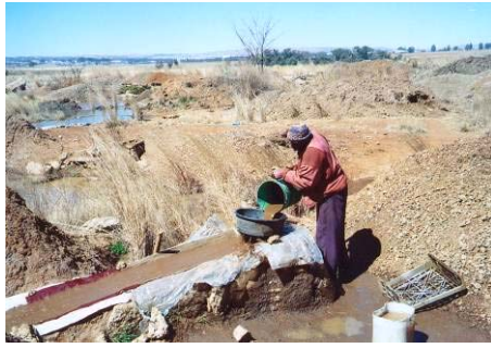
Fig. 4.2 - Hand fed sluice in South Africa
