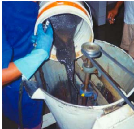
Fig. 5.3 – Miner introducing concentrate into a high speed blender--this is very inefficient because the high speed flours the mercury
