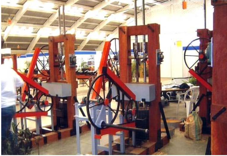
Fig. 3.23 – Hand stamp mill made in Zimbabwe. One and two stamp models are available.
