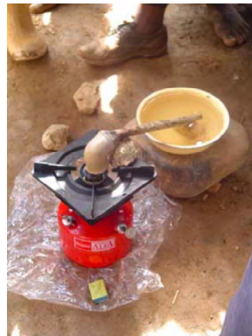
Fig. 5.39 - Heating an RHYP pipe retort with a kerosene stove.
