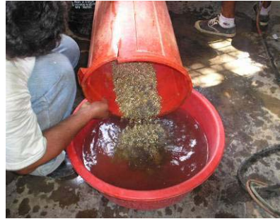
Fig. 6.8 – Zinc shavings are leached with sulphuric acid and gold is left behind.
