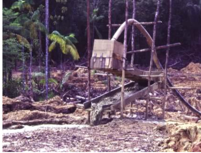
Fig. 4.8 - Pump-fed zigzag sluice in Suriname
