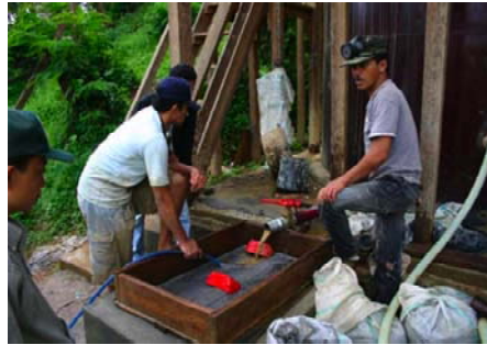
Fig. 6.9 - Recovery of gold loaded carbon using a screen.
