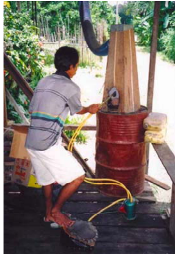
Fig. 5.36 - Indonesian miners burning amalgam using a foot pump-gasoline-air torch
