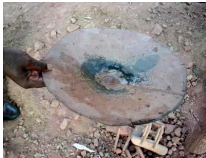
Fig. 4.20 - Riveted shallow batea made of sheet metal (Brazil)
