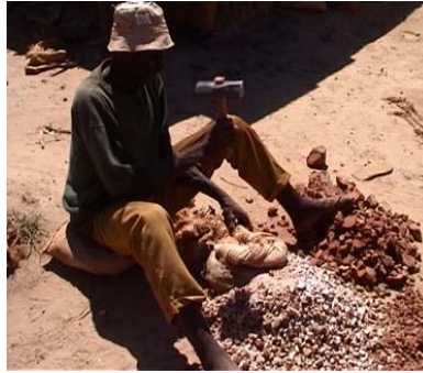
Fig. 3.21 – Miner in Tanzania using a cloth Hessian ring around the rock to protect his hands when crushing with a hammer
