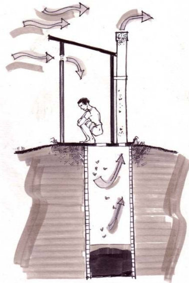
Fig. 10.5 - Ventilated pit latrines (VIP) are host to only 1% of the flies that are attracted to simple pit latrines. (Illustration L. Pevick)
