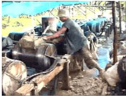
Fig. 3.17 – Series of small belt-driven ball mills in Sulawesi, Indonesia
