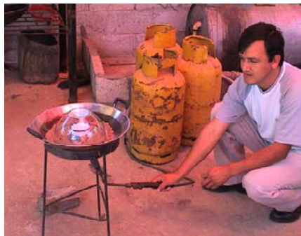
Fig. 5.29 – Ecuadorian miner using the kitchen-bowl retort with a torch
