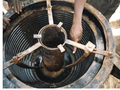
Fig. 4.14 – Rubber cone with ribs (ABJ centrifuge)
