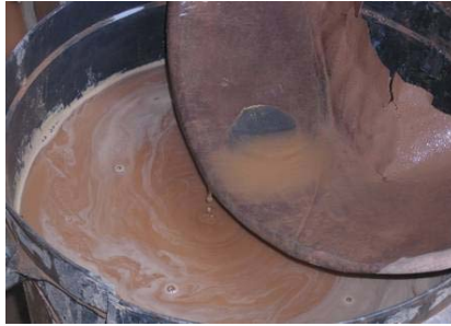
Fig. 4.16 - Miners can capture fine gold even in a very worn out pans (Tanzania)
