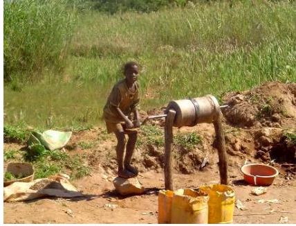
Fig. 3.25 - Small manual ball mill used in Mozambique
