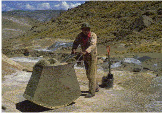
Fig. 3.27 - Quimbaleta filled with stones on steel plate (photo M. Priester)
