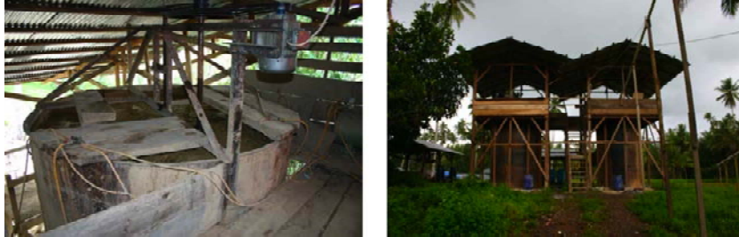
Fig. 6.5 – Tanks of gold cyanidation in North Sulawesi, Indonesia
