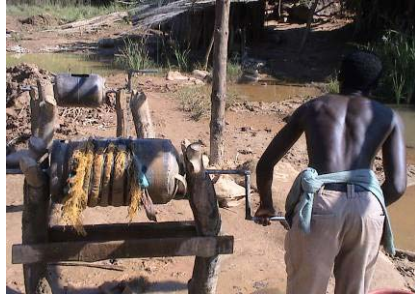
Fig. 2.5 - Manual ball mill made of LPG tank (Mozambique)
