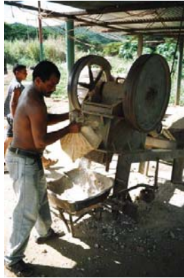
Fig. 3.4 – Venezuelan miner feeding a small jaw crusher
