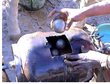
Fig. 3.26 – Loading steel balls into a manual ball mill
