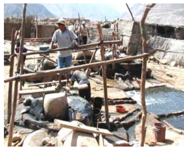
Fig. 3.29 – Quimbaleta operated by foot (photo A.J. Gunson)
