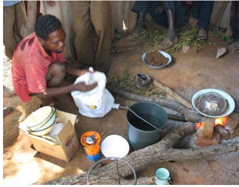
Fig. 5.40 – Operating a “mvuto” that blows air into a bonfire with a kitchen-bowl retort (Zimbabwe)
