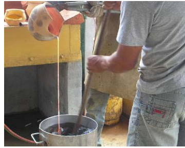
Fig. 6.10 - Pouring of smelt product into water to obtain fine droplets of gold before extracting silver
