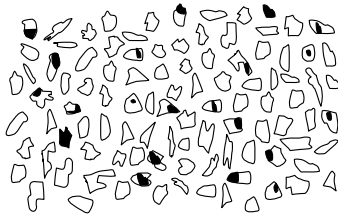
Fig. 2.3 – Example of an ore with poor liberation. Gold (dark) is still mostly attached to the gangue (white)
