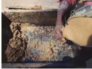
Fig. 4.5 - Feed box for hand fed sluice: mixing ore with water
