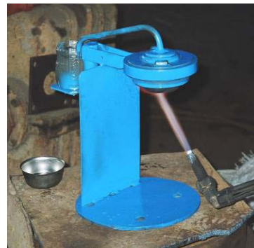
Fig. 5.19 – Venezuelan retort in operation (extra stainless steel crucible shown at left).
