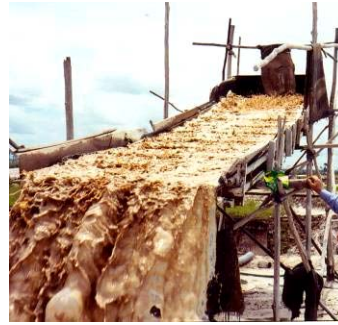
Fig. 4.3 - Monitor pump fed sluice in Indonesia. Note the turbulent flow which limits recovery of fine gold
