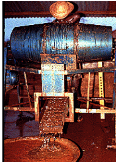
Fig. 5.1 – Miner discharging an amalgamation drum on a sluice box
