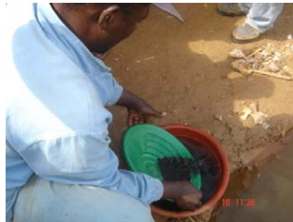
Fig. 4.21 - North American plastic pan with riffles in the side (Mozambique)
