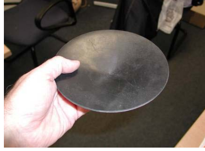
Fig. 4.22 - Small rubber coated cone-shaped batea for testing ore (Peru)
