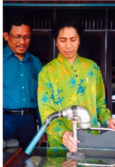
Fig. 5.21 – Indonesian version of the RHYP retort with a 2” crucible
