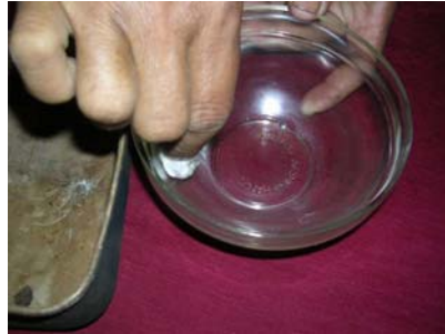
Fig. 5.34 – Miner in Lao PDR: recovering mercury from a glass bowl retort using cotton
