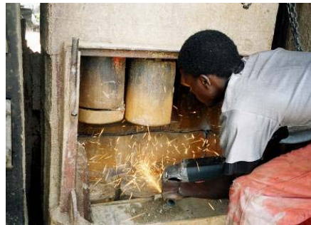
Fig. 3.12 – Miner grinding the base of stamps inside a mill
