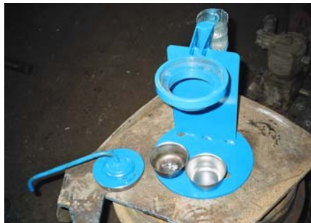
Fig. 5.18 – Venezuelan retort; a low cost stainless steel crucible bowl fits into the opening.
