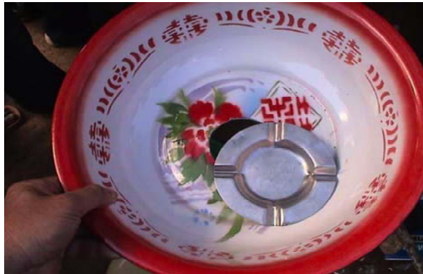
Fig. 5.32 – Stainless steel ashtray used as crucible in the kitchen-bowl retort
