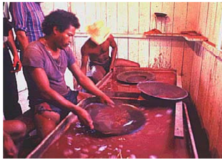
Fig. 5.6 - Miner separating the amalgam from the heavy minerals by panning in a water box
