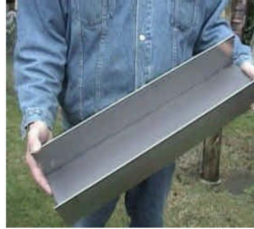
Fig. 4.11 – Cleangold magnetic sluice
